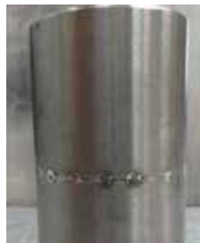
Pipe butt weld Ø 31,75 x 2 mm.
