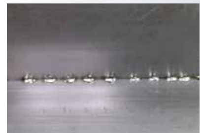
Corner spot welding thickness 0,6 mm.
