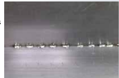
Corner spot welding thickness 0,6 mm
