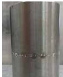
Pipe butt weld Ø 31.75 x 2 mm
