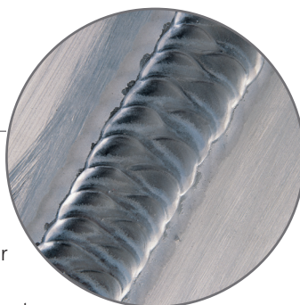
Alumaxx® Plus TIG-stomplas in 10mm dikke 4140 aluminiumlegering met Alumaxx® Plus
